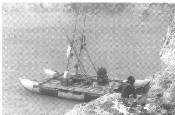
Fig. 4 The catamaran working on the lake. Note a winch on the deck to take water samples at various depth
