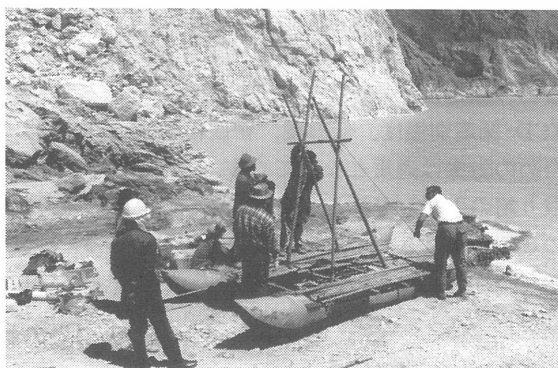
Fig.2 A catamaran being constructed on the shore of Kawah Ijen crater lake. The deck of the boat was made of bamboo sticks
