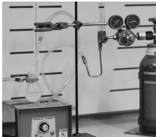
Fig. 2 Bubbling of H 2 S for the hot spring water solution containing inorganic salts and formaldehyde.
